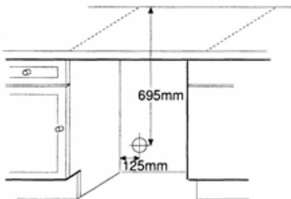
If the through the wall vent is to be positioned other than behind the dryer, the vent hose should be positioned at floor level and through adjacent side panel to a relevant position. The plinth must be cut-out to accommodate the air vent grill at the bottom front of the tumble dryer.
