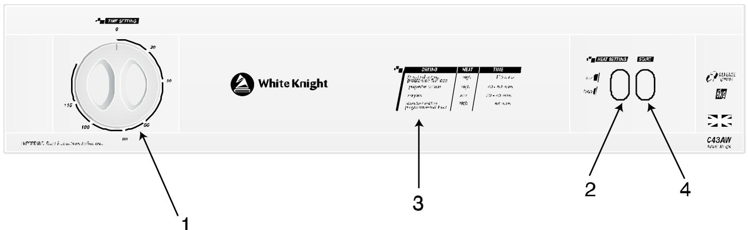
1. The Timer                      Select the drying time from the recommendations shown on the control panel (3). Turn the timer knob clockwise for required drying time.
